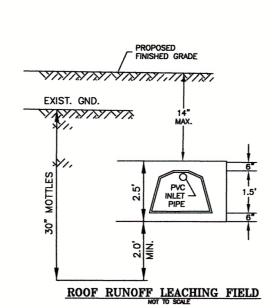
1. THIS ROOF RUNOFF LEACHING SYSTEM WAS DESIGNED TO CAPTURE 1.0-INCHES OF RUNOFF
