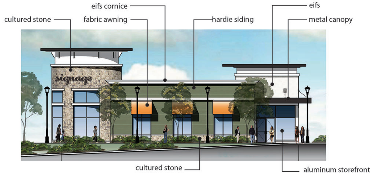
Side Elevation at Building O
