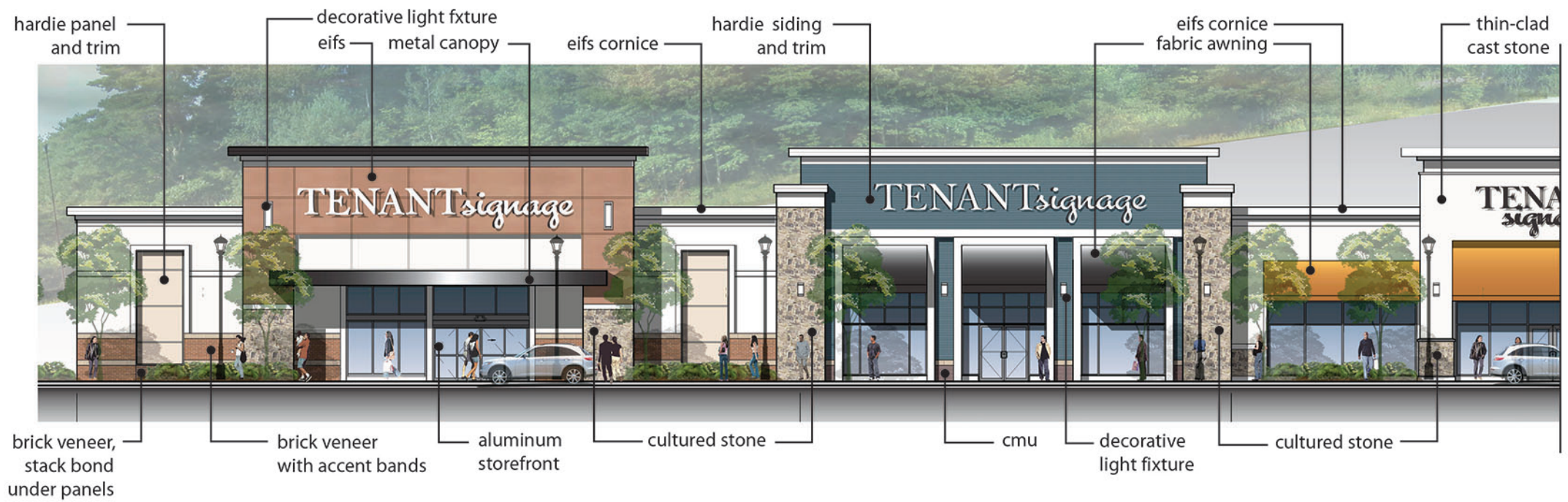
Partial Front Elevation at Building E-I
