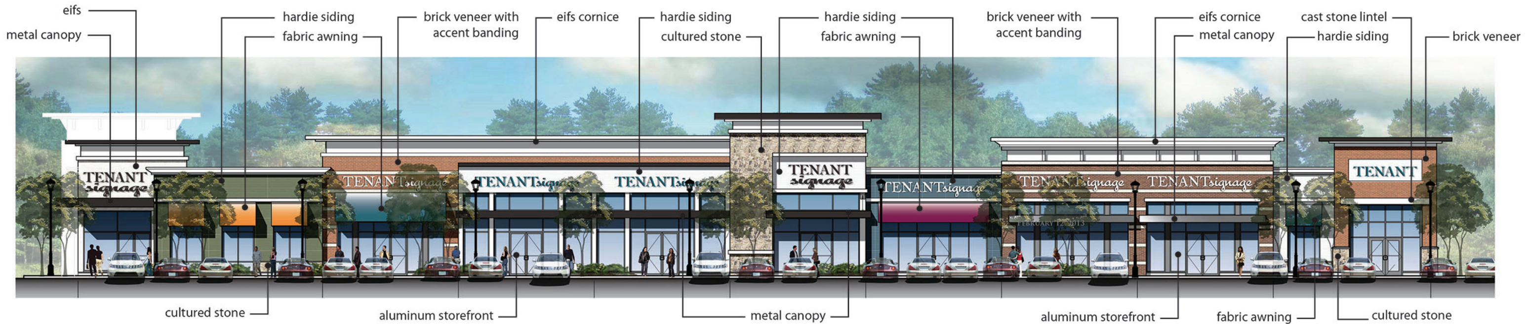
Front Elevation at Building O
