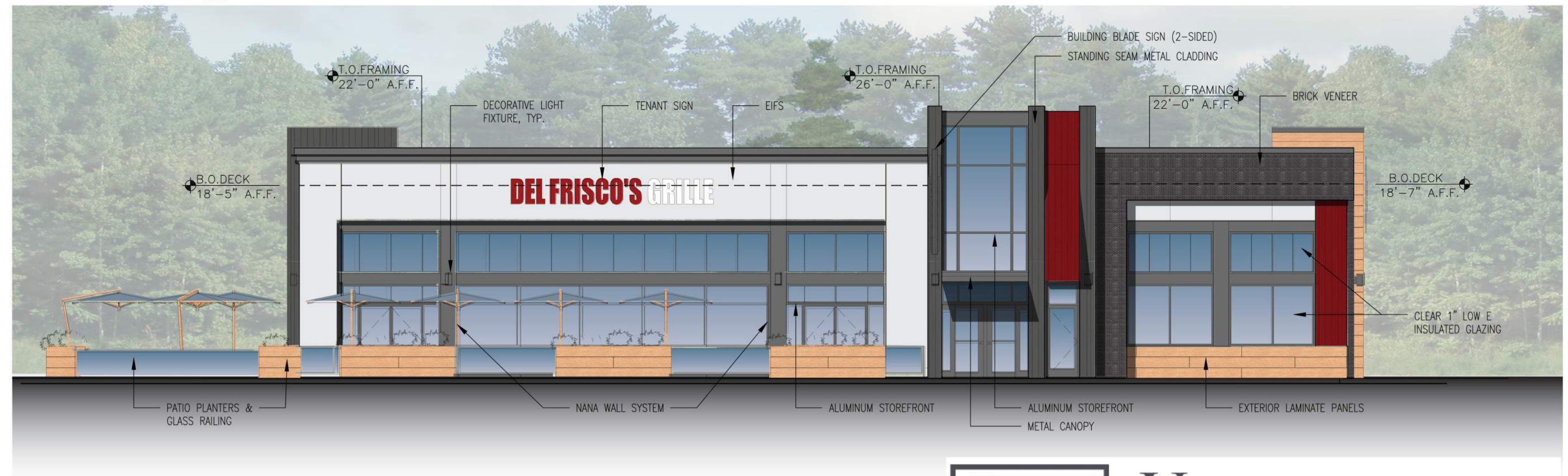
4 Front Elevation (Parking Lot Side)
