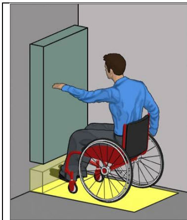
Objects that provide clearance for toes can overlap a portion of the clear floor space.
