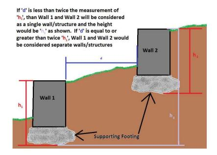
6) Add a new definition for "Combined Wall and Fence Height" to read as follows, including illustration:
