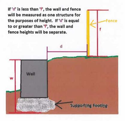
6) Add a new definition for "Combined Wall and Fence Height" to read as follows, including illustration:
