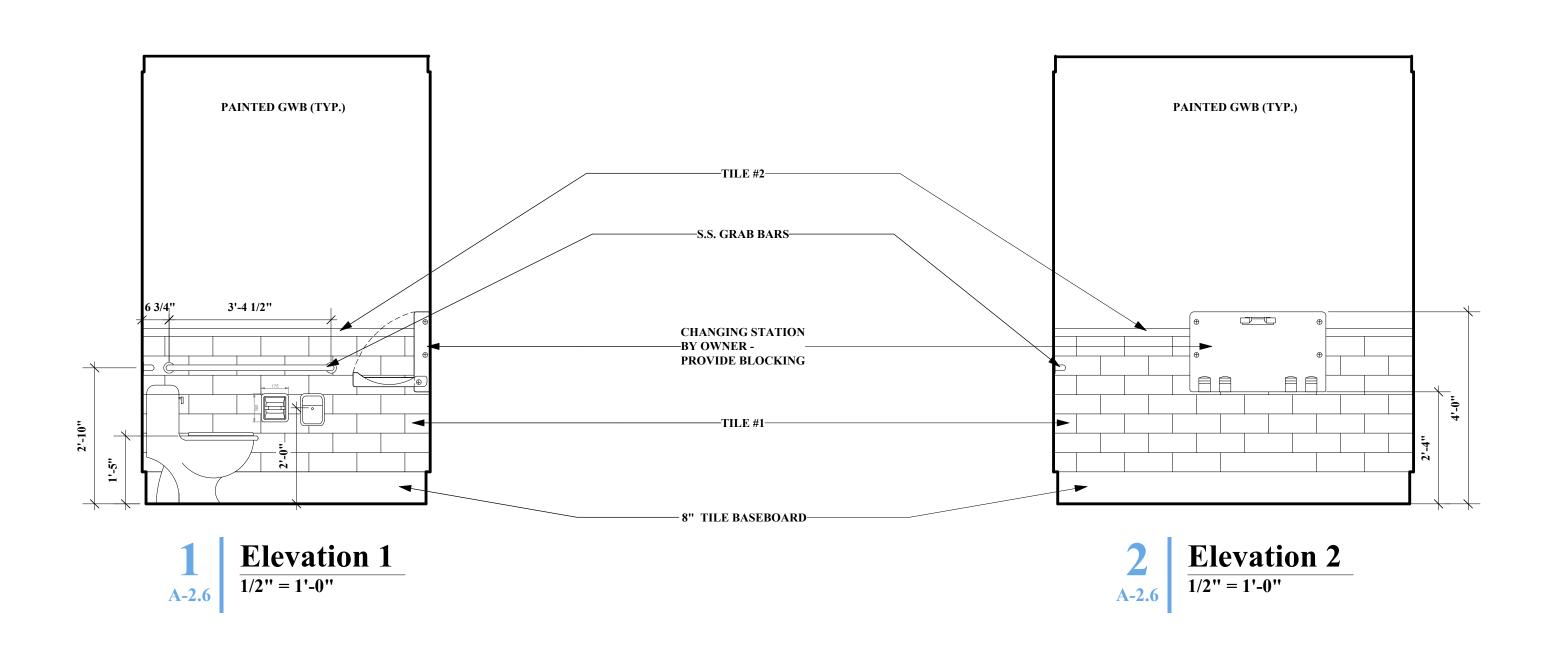
ALL ACCESSORIES ARE TO BE NAAMM ARCHITECT, USE ONLY CONCEALED FASTENERS AND PROVIDE SOLID BLOCKING TO ALLOW FOR 250 POUND LOAD ACTING ON ANY ACCESSORY.
