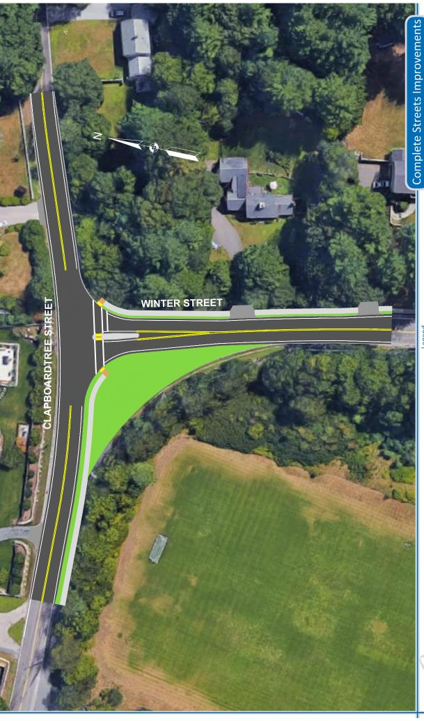
Legend = Pavement Resurfacing= Cement Concrete Sidewalk
